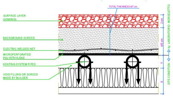
THE FILLING ON THE HEATING SYSTEM, INDICATED FLUSH WITH THE PIPES SCAN BE THICKER ACCORDING TO THE TOTAL SPACE AVAILABLE ON SITE.
